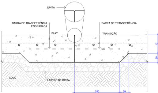
DETALHE JUNTA CONCRETAGEM
